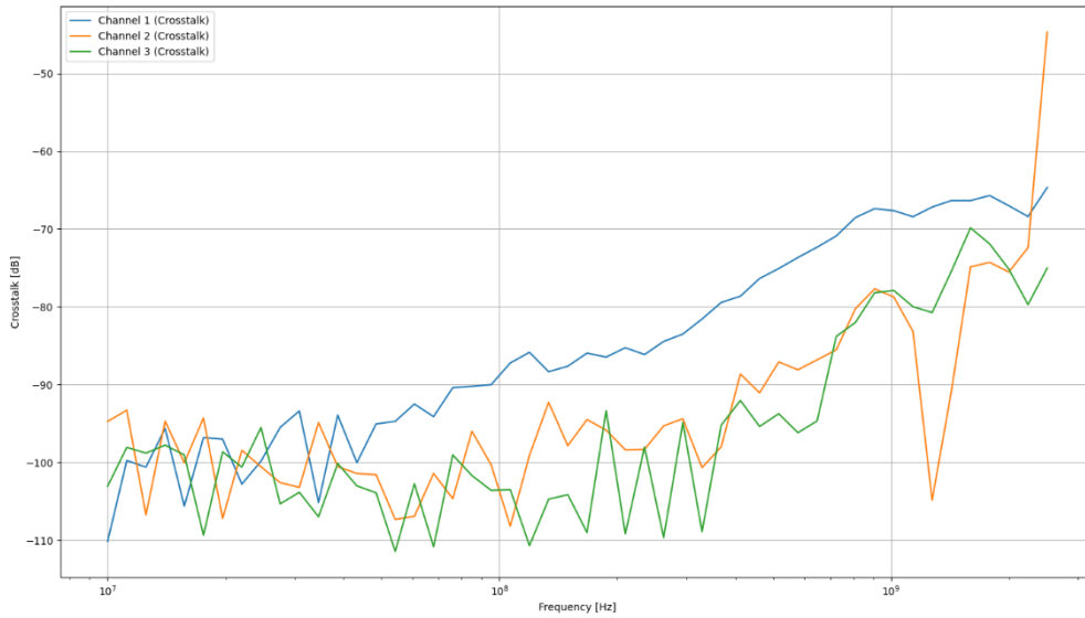
Figure 5 Typical crosstalk in 4-channel mode. Channel A to B, C and D.
